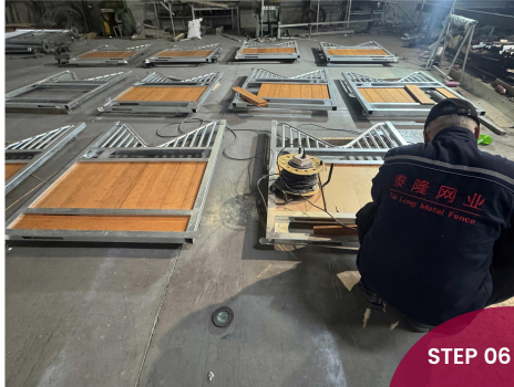
Bamboo And Wood Installation
